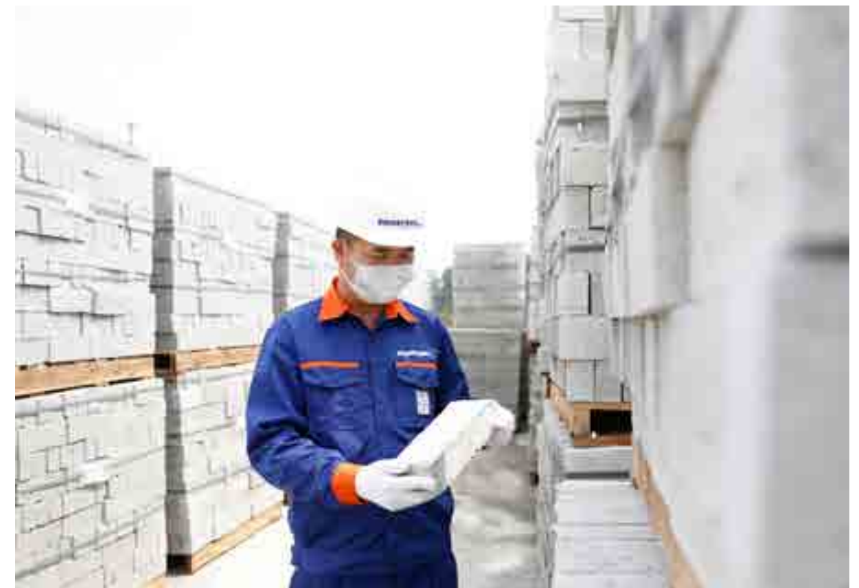
Sludge used as input for unburnt bricks
