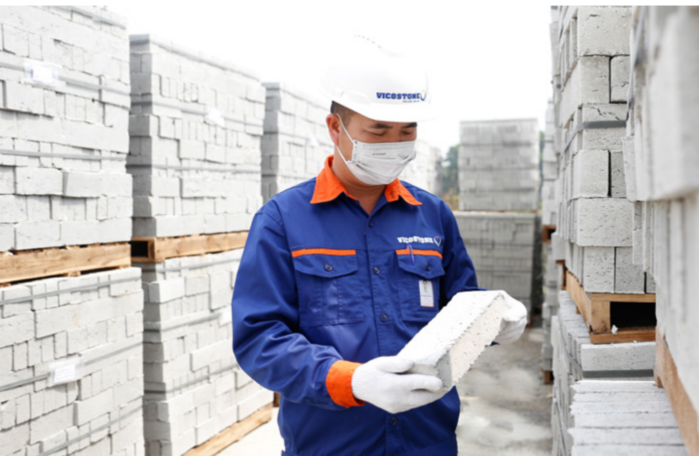
Unburnt bricks made from sludge that is disposed of the production
